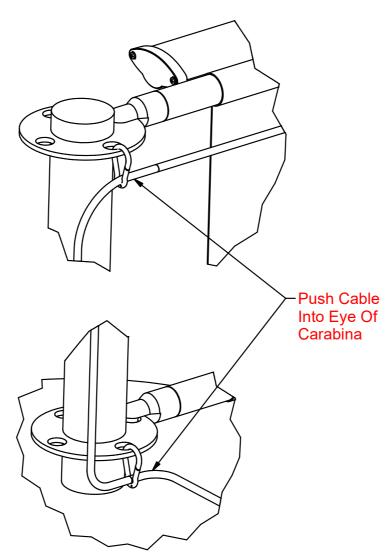
4) When a gangway is present use extra long link cable between the gap. Fix cable top and bottom of post ,ensure cable to push into carabina clips. Cut cable cover to length and cover cable.
